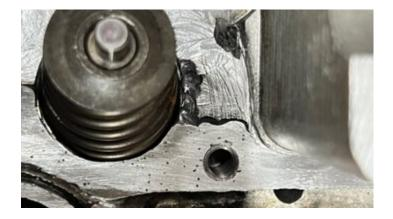
The background is: Cylinder heads in Porsche vehicles are often destroyed by cracking as a result of excessive heat input. This results in further engine damage. We notice this again and again in connection with engine repairs.
